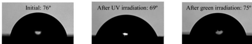
Fig. 4. WCA of a water drop of volume 3 \mu\text{l} on flat photochromic polymer surface before and after UV-green laser irradiation. (5% wt of SP in PEMMA, \lambda_{UV}=308\text{ nm} , F_{UV}=40\text{ mJ cm}^{-2} , \lambda_{green}=532\text{ nm} , F_{green}=45\text{ mJ cm}^{-2} ) (Athanasidou et al 2006a)
